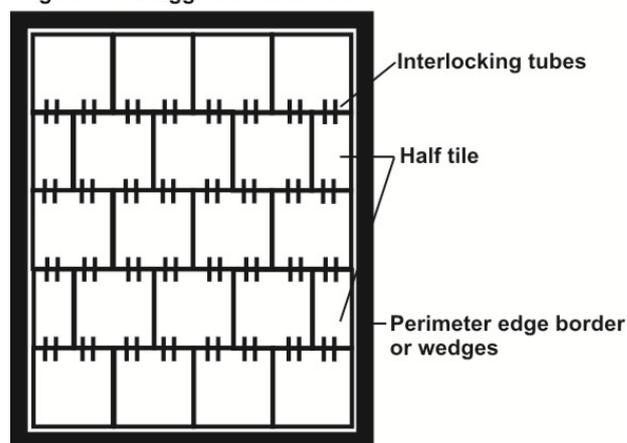
**The correct installation of THE TYRED FLOORING COMPANY Rubber Tiles is a staggered pattern to ensure proper alignment, a tighter fit, and reduction of vandalism.**
