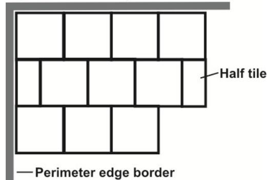
**THE CORRECT INSTALLATION OF TYRED FLOORING RUBBER TILES IS A STAGGERED PATTERN TO ENSURE PROPER ALIGNMENT, A TIGHTER FIT, AND REDUCTION OF VANDALISM.**
